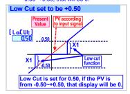
2. If set the negative value (X2) here to display "X2" which it expressed to be low-cut the PV that it's under the X2 setting value;
