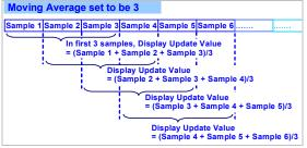
Remark: The higher moving average setting wouldn't cause the response time of Relay and Analogue output slower after first 3 samples.
