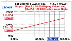
The range between [ AaH5] and [ AaL5] should be over 20% of span at least; otherwise, it will be got less resolution of analogue output.
