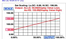
The range between RoH5 and RoL5 should be over 20% of span at least; otherwise, it will be got less resolution of analogue output.
