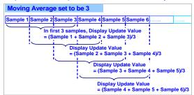
Remark: The higher moving average setting wouldn't cause the response time of Relay and Analogue output slower after first 3 samples. Digital filter: The digital filter can reduce the magnetic noise in field.
